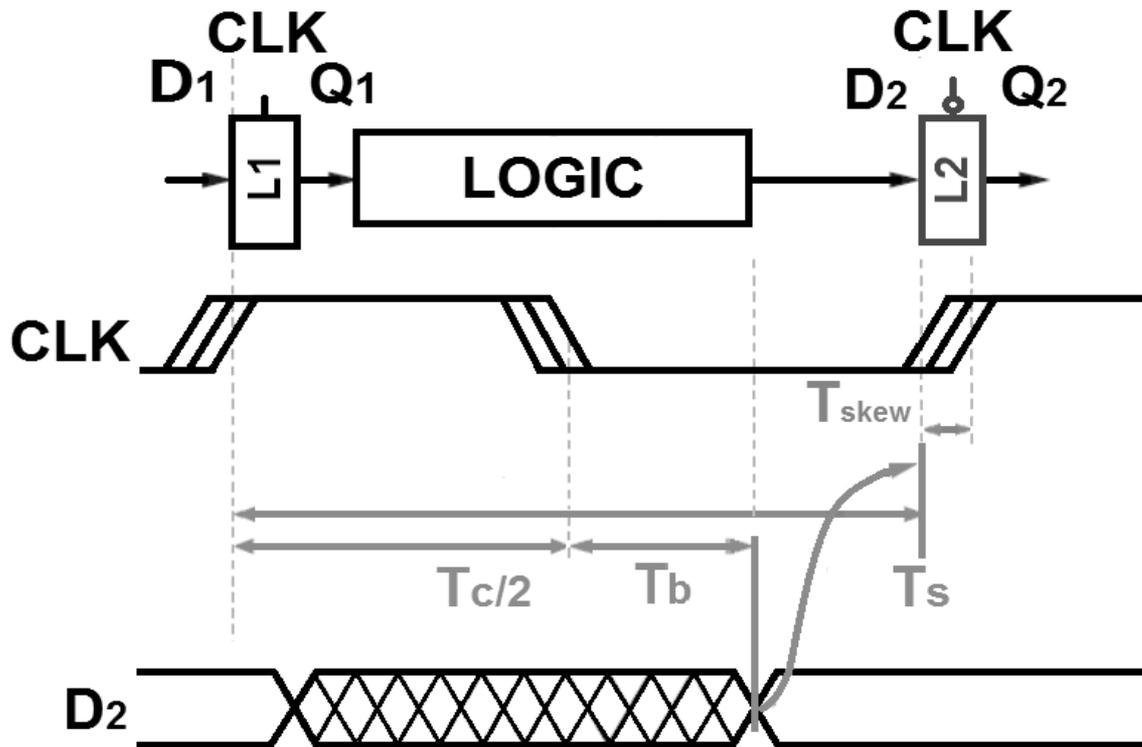
$$T_b \leq T_c/2 - (T_s + T_{skew}) \quad [2]$$
