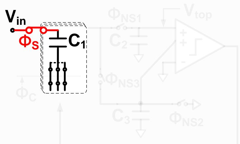
Get half top voltage,  $V_{C3} = V_{top} (n-1)/2$ ; Sampling input,  $V_{in}(n)$ ;
