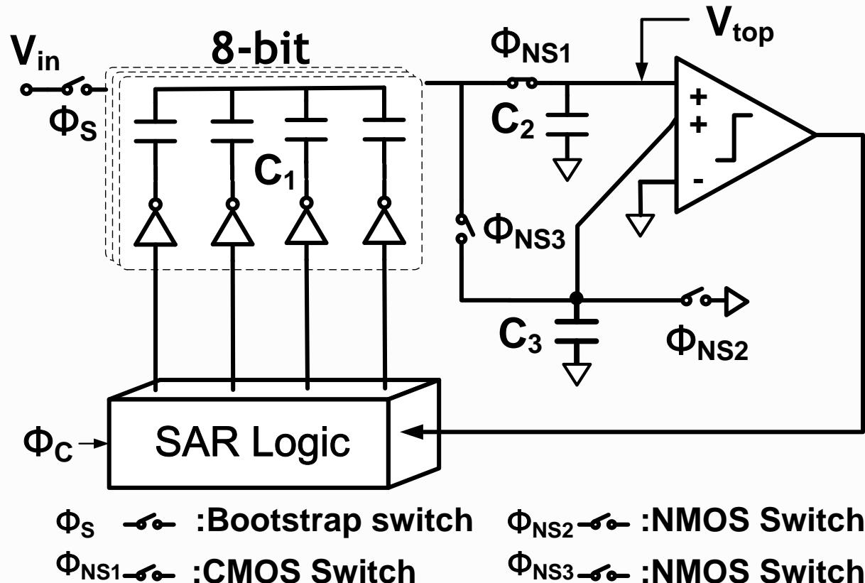
Asynchronous logic; 8-bit C-DAC
