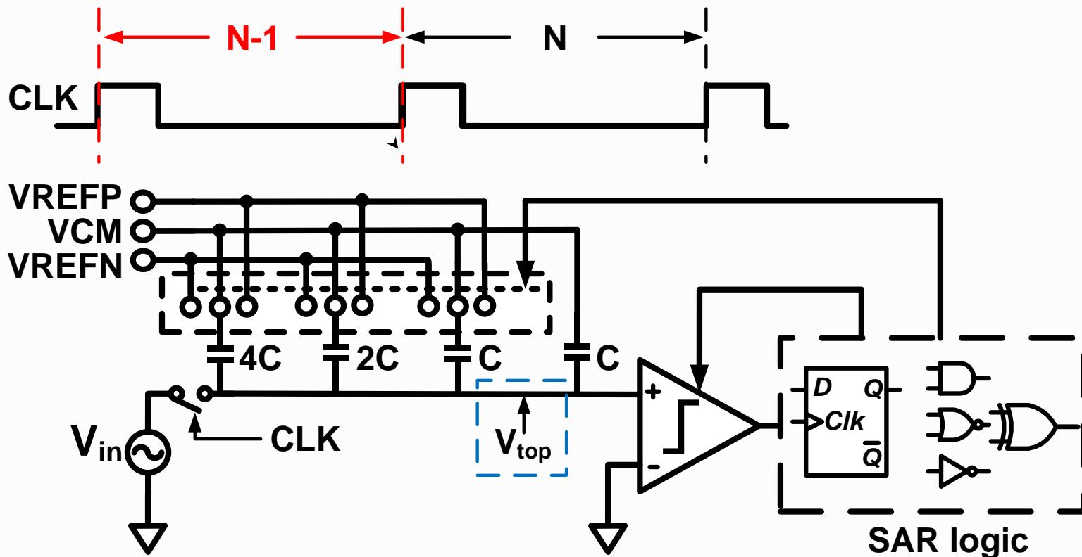
After conversion @ N-1, residue  $V_{top}(N-1) = X_{SAR,in}(N-1) - Y(N-1)$
