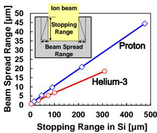
**Fig. 4:** Calculated beam spread range with respect to ion stopping range in silicon by using TRIM calculating 10 thousand times with 95% ion falling within the range.
