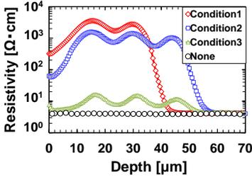
**Fig. 3:** Substrate resistivity variation as a function of depth from the surface of Si wafer with various conditions (Table 1).
