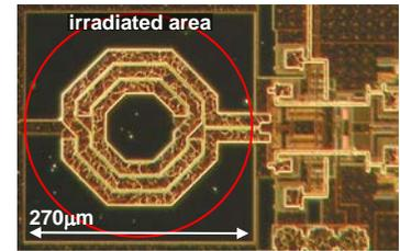
**Fig. 11:** VCO chip photo with the irradiated area (condition #2). The active area covered by the aluminum mask.
