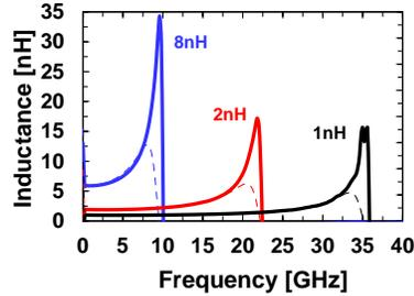
**Fig. 6:** Inductance (1nH, 2nH, and 8nH) with (solid lines) and without (dotted lines) the helium-3 bombardment. Condition #2 in Table 1 is applied.
