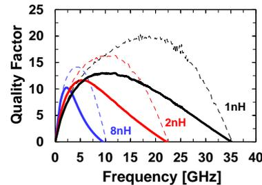
**Fig. 7:** Quality factor of inductors (1nH, 2nH, and 8nH) with (solid lines) and without (dotted lines) the helium-3 bombardment. Condition #2 in Table 1 is applied. The Q improvement ratios are 36% (Q=10.3 to 14.1), 38% (Q=11.6 to 16.3), and 54% (Q=13.0 to 20) for 8nH, 2nH, and 1nH inductors, respectively. The peak frequencies are shifted to higher while the self-resonance frequencies are not changed.
