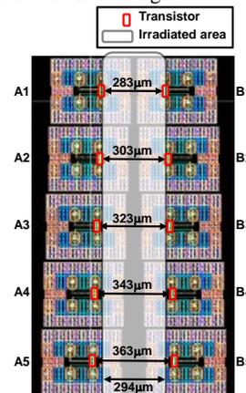
**Fig. 8:** TEG structure for evaluating transistor damage from the bombardment.
