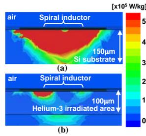
**Fig. 5:** Electromagnetic simulation results of specific absorption rate (SAR) wo (a) / w (b) 100μm-depth helium-3 bombardment, which contributes to drastically reducing the absorption into the lossy Si substrate.
