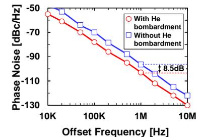
**Fig. 12:** Measured phase noise with/without the bombardment. An 8.5-dB improvement is achieved with the same 5.6-mW power consumption.
