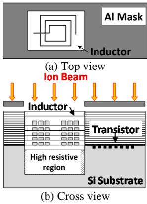
**Fig. 1:** Helium-3 bombardment process. For covering active areas, a 0.5mm-thick aluminum plate is used as a mask from the irradiation.
