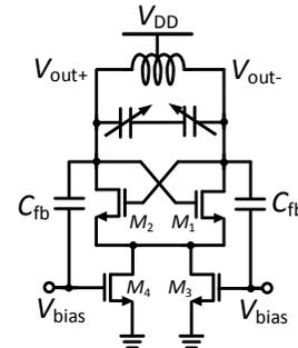
**Fig. 10:** Circuit schematic of tail-feedback voltage control oscillator (VCO), designed for 8-GHz oscillation. A 1-nH inductor is used.
