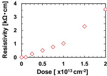
**Fig. 2:** Substrate resistivity with dose amount.
