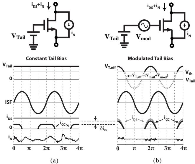
Fig.3. Tail noise suppression using modulated tail bias.
