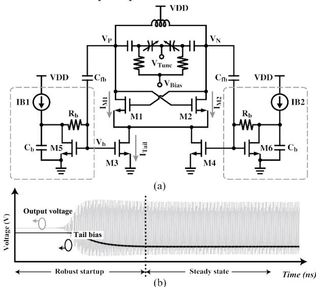
Fig.4. Proposed tail-current modulated VCO with adaptive startup (a) and simulated waveforms of interest (b).
