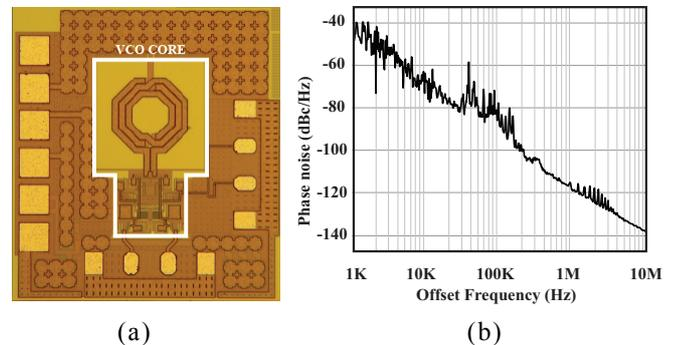
Fig.5. Chip micrograph of the proposed VCO (a) and the measured phase noise plot (b).
