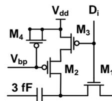
Fig. 3. Proposed capacitor-switch unit.
