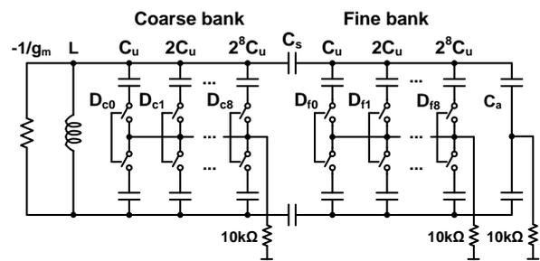
Fig. 2. Equivalent model of the DCO with the topology of proposed coarse and fine banks.
