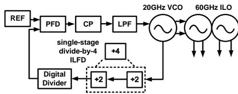
(b) Sub-harmonic injection based on 20GHz PLL
