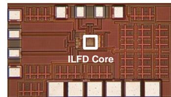
Fig.4. Chip Micrograph of the proposed ILFD
