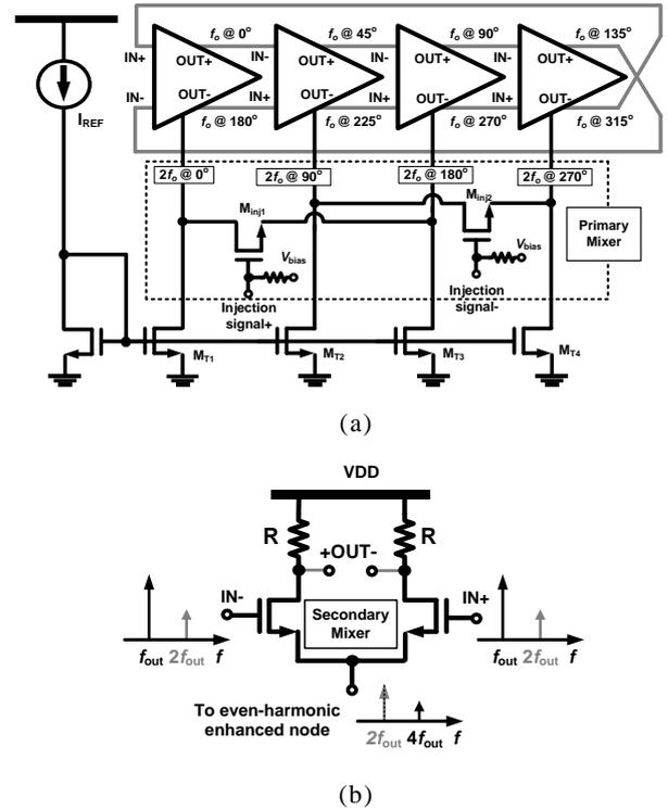
Fig.3. Detailed circuit schematic of the proposed (a) dual-step-mixing ILFD and (b) its delay cell
