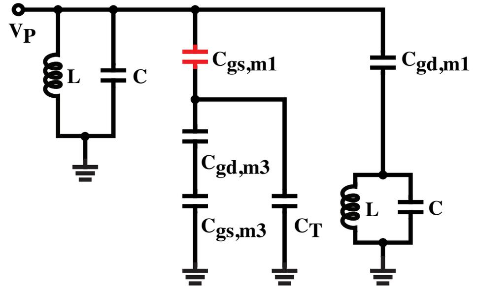
Conventional Class-C equivalent circuit
