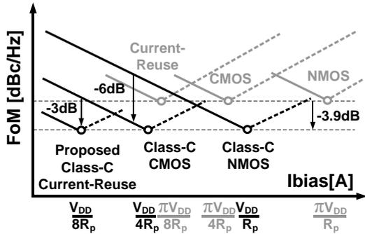
Fig.1. Theoretical FoM limit of conventional class of VCOs and its corresponding Class-C VCOs.
