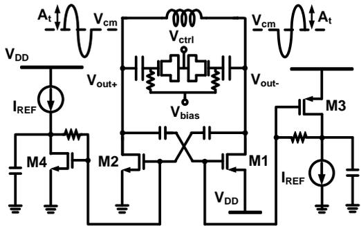
Fig.2. Proposed swing-enhanced current-reuse class-C VCO using dynamic bias control circuits
