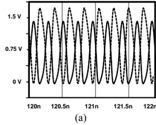
Fig.5 Output amplitude of current-reuse VCO (a) without and (b) with dynamic bias control circuits.
