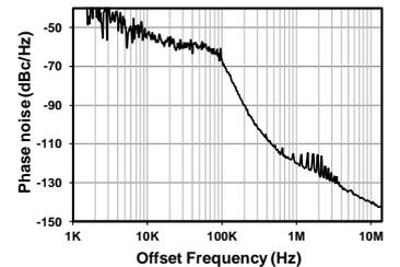
Fig.7. Measured phase noise plot at 4.63GHz
