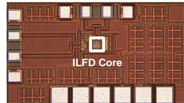
Fig.4. Chip Micrograph of the proposed ILFD
