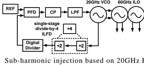
Fig.1. 60GHz frequency synthesizers proposed in [1],[2]
