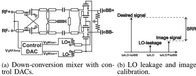
Fig. 3. I/Q mismatch calibration.
