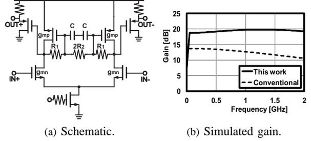
Fig. 5. Gain peaking amplifier in Rx baseband.
