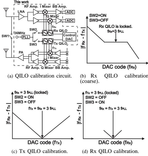
Fig. 2. Proposed QILO calibration.
