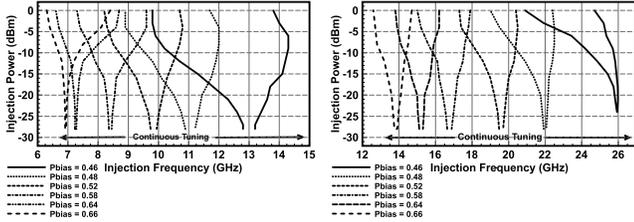
Fig. 4. Divide-by-4 locking and operation range with input applied to divide-by-4 terminals (left) and divide-by-8 locking and operation range with input applied to divide-by-8 terminals of the divide-by-8 PMILFD
