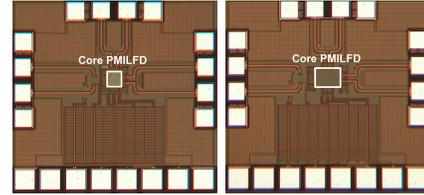
Fig. 5. Divide-by-4 PMILFD (on the left) and divide-by-8 PMILFD (on the right) chip photos
