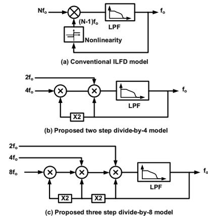
Fig. 1. ILFD models: (a) Conventional (b) Proposed two-step divide-by-4 (c) Proposed three-step divide-by-8
