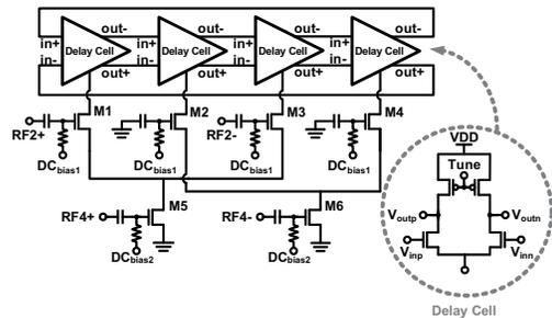
Fig. 2. Proposed PMILFD divide-by-4 circuit
