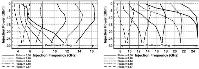
Fig. 3. Divide-by-2 locking and operation range with input applied to RF2 terminals (left) and divide-by-4 locking and operation range with input applied to RF4 terminals (right) of the divide-by-4 PMILFD
