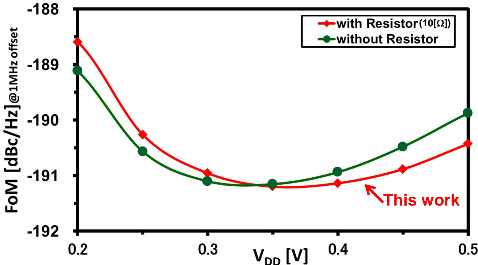
$$\text{FoM} = \mathcal{L}(f_{\text{offset}}) - 20 \log \left( \frac{f_0}{f_{\text{offset}}} \right) + 10 \log \left( \frac{P_{\text{DC}}}{1 \text{ [mW]}} \right)$$
