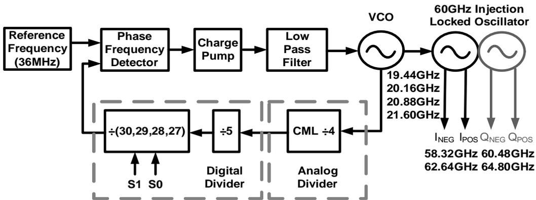
Fig.4: 60GHz Frequency synthesizer using quadrature injection-locked oscillator (QILO)
