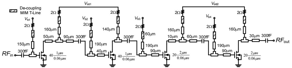
Fig.1: Schematic of 60GHz low-noise amplifier
