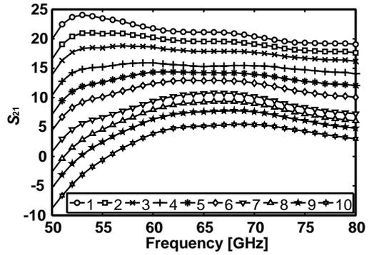
Fig.3: Gain control of LNA
