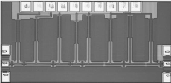
Fig.2: Chip microphoto of LNA
