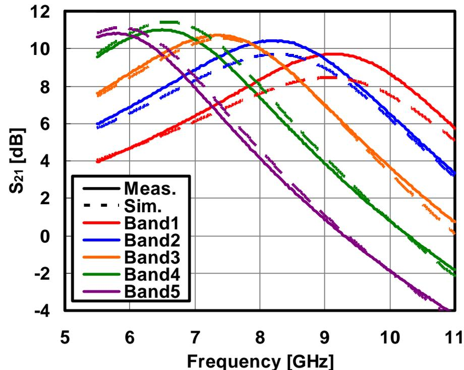
■ Measurement results are slightly shifted to lower frequency due to model inaccuracy
