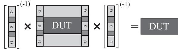
Fig. 3 L-2L De-embedding procedure.
