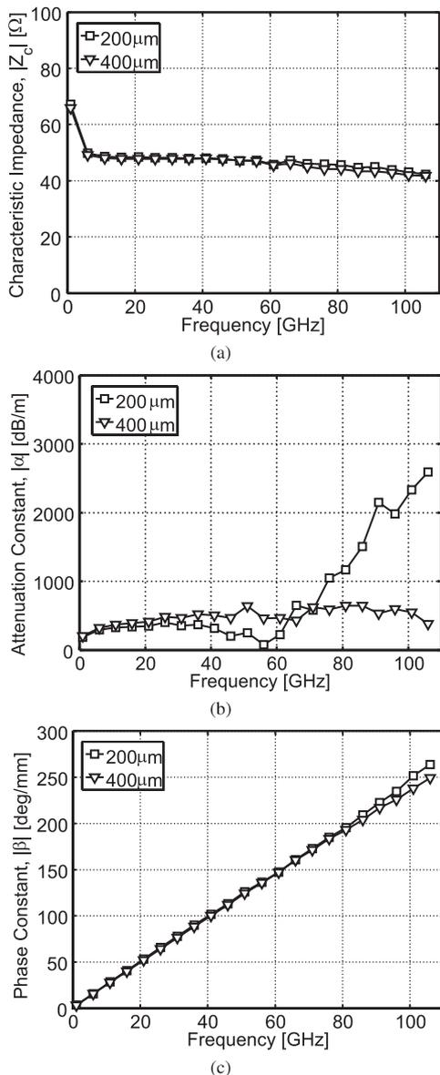
**Fig. 8** Through-only de-embedding method for 200- $\mu\text{m}$  and 400- $\mu\text{m}$  CPWs with two-metal ground. (a) Characteristic impedance. (b) Attenuation constant. (c) Phase constant.
