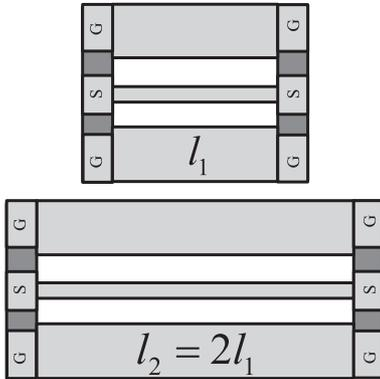
Fig. 1 L-2L through-line test structures.
