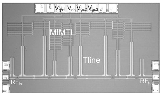
Fig. 15 Micrograph of the four-stage PA.
