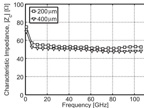
Fig. 7 Open-short de-embedding method for the characteristic impedance of  $200\text{-}\mu\text{m}$  and  $400\text{-}\mu\text{m}$  CPWs with two-metal ground.
