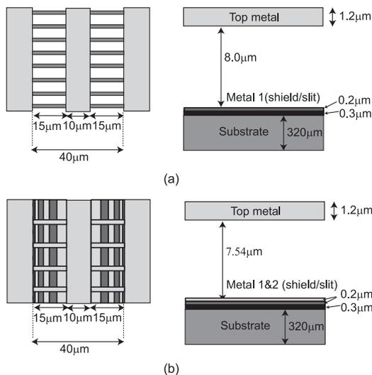
Fig. 5 Cross section of the transmission line. (a) Slow-wave coplanar waveguide (SWCPW). (b) CPW with two-metal ground.
