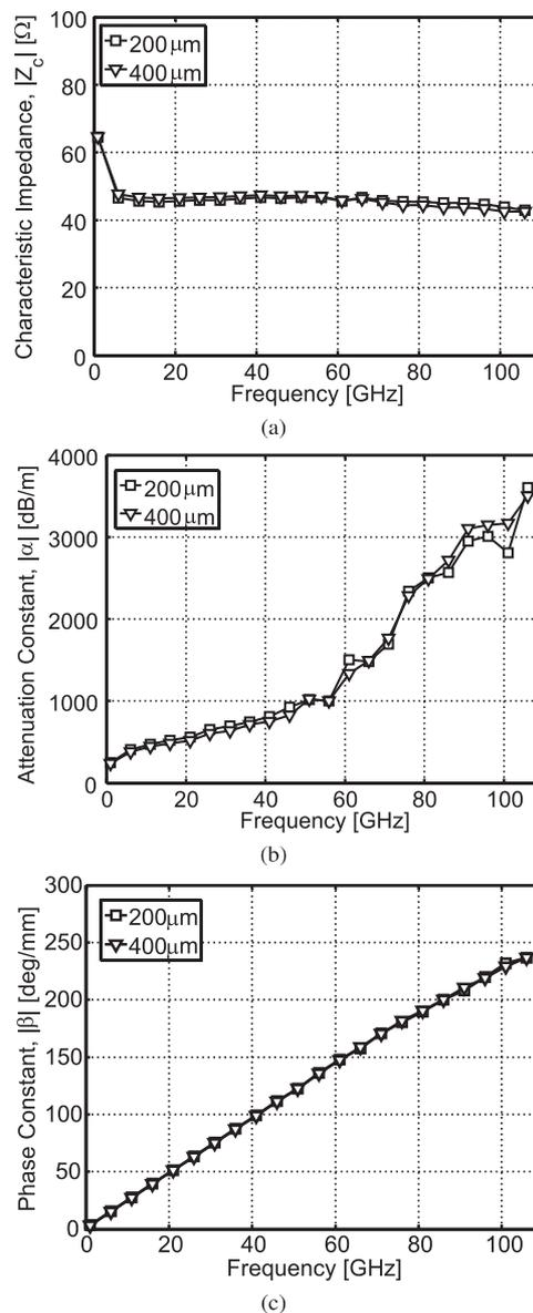
**Fig. 9** L-2L through-line de-embedding method for 200- $\mu\text{m}$  and 400- $\mu\text{m}$  CPWs with two-metal ground. (a) Characteristic impedance. (b) Attenuation constant. (c) Phase constant.
