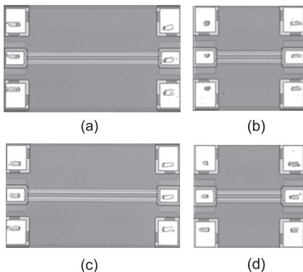
Fig. 6 Micrograph of the transmission lines. (a)  $400\text{-}\mu\text{m}$  Slow-wave coplanar waveguide (SWCPW). (b)  $200\text{-}\mu\text{m}$  SWCPW. (c)  $400\text{-}\mu\text{m}$  CPW with two-metal ground. (d)  $200\text{-}\mu\text{m}$  CPW with two-metal ground.
