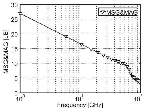
**Fig. 11** Measured maximum stable gain or maximum available gain of a transistor at a  $V_{gs}$  of 0.8 V and a  $V_{ds}$  of 1.2 V.
