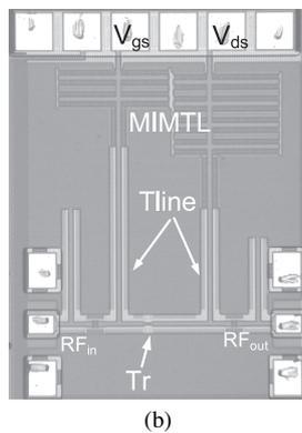
**Fig. 12** Schematic and micrograph of the one-stage amplifier.
