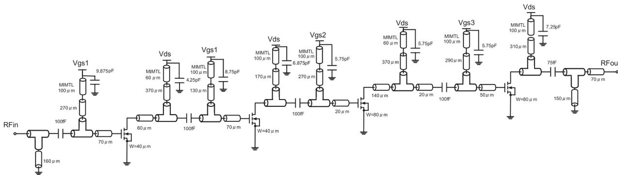
Fig. 14 Circuit schematic of the four-stage power amplifier.
