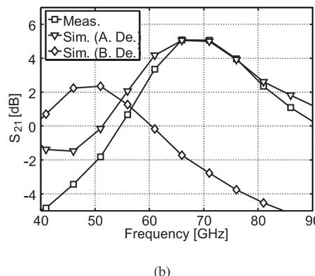
**Fig. 13** Comparison between the measured and simulated results of the one-stage amplifier at a  $V_{gs}$  of 0.8 V and a  $V_{ds}$  of 1.2 V. (a)  $S_{11}$  and  $S_{22}$  with markers at 67 GHz. (b)  $S_{21}$ .
