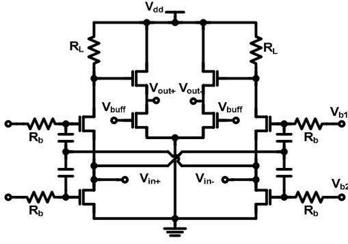
Fig. 6 Schematic of the low noise amplifier
