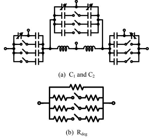
Fig. 4 Detail of the  $C_1$ ,  $C_2$ , and  $R_{deg}$
