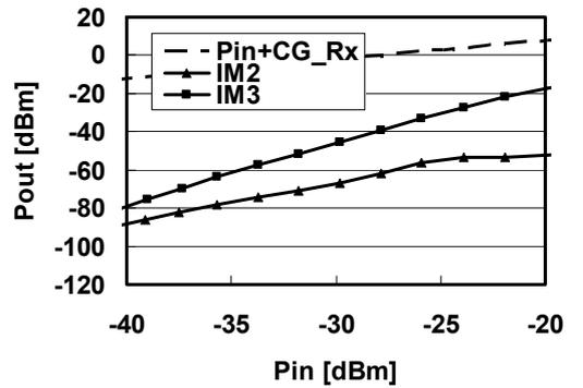
Fig. 11 Measured IM<sub>2</sub> and IM<sub>3</sub> at 1.5GHz
