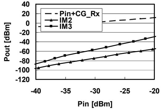
Fig. 10 Measured IM<sub>2</sub> and IM<sub>3</sub> at 0.8GHz
