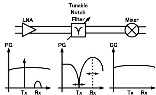
Fig. 1 Receiver architecture
