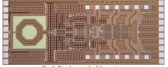
Fig. 8 Die photograph of the receiver
