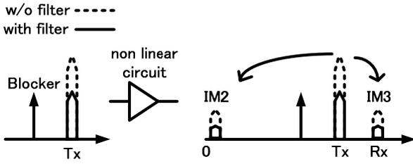
Fig. 2 Tx and IM3 suppression by notch filter
