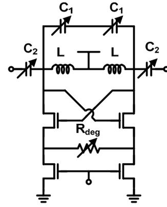
Fig. 3 Schematic of the proposed tunable notch filter
