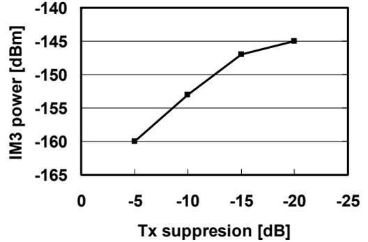
Fig. 5 Trade-off between the Tx suppression and linearity
