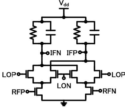
Fig. 7 Schematic of the mixer
