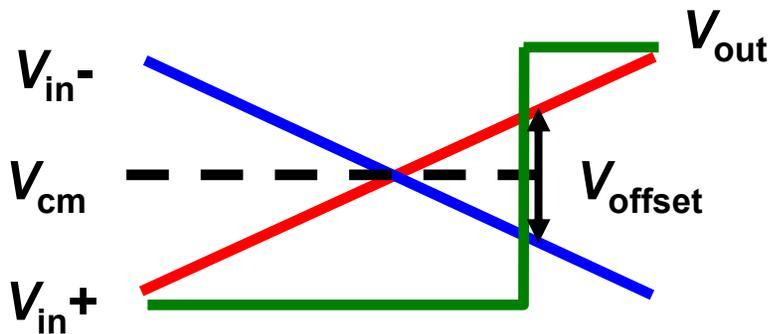
The offset voltage is the input voltage at the point that output changes from low to high.
