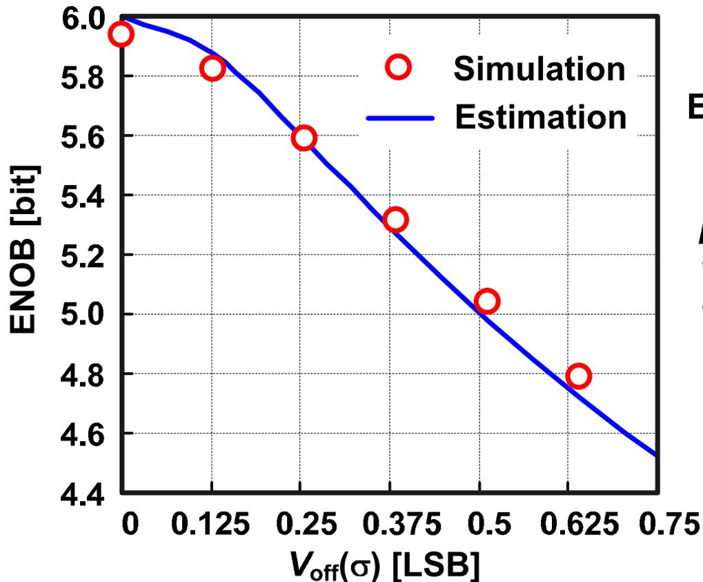
$$\text{ENOB} = N - \frac{1}{2} \log_2 \left[ 1 + 12 \left( \frac{V_{\text{off}}(\sigma)}{V_q} \right)^2 \right]$$
