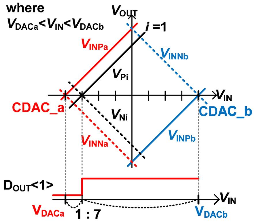
$$V_{Pi} = \frac{(8 - i)V_{INPa} + iV_{INPb}}{8}, \quad V_{Ni} = \frac{(8 - i)V_{INNa} + iV_{INNb}}{8}$$
