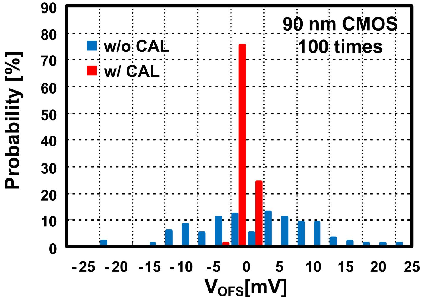
Offset variation is reduced **from  $9\text{mV}_{\text{RMS}}$  to  $0.9\text{mV}_{\text{RMS}}$ .**
