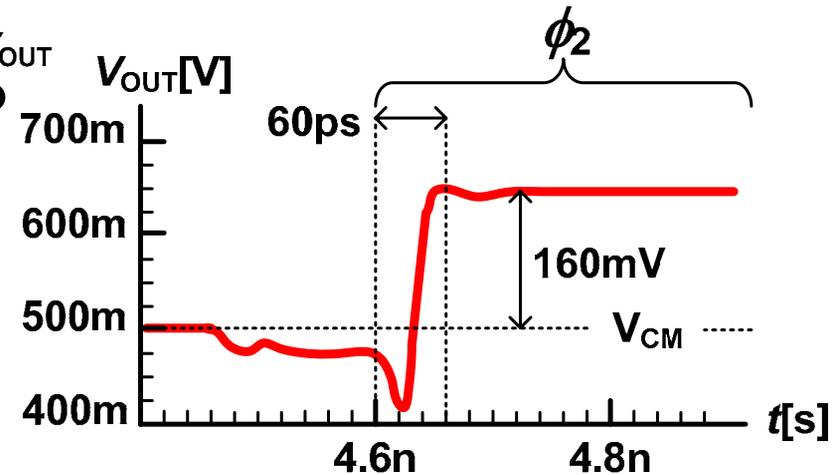
$$V_{OUT} = \frac{16C_U}{16C_U + C_P} (V_{IN} - V_{DAC})$$
