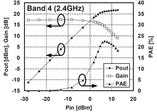
Fig. 7. Measured output power, gain, and power added efficiency versus input power at band 4 (2.4GHz).
