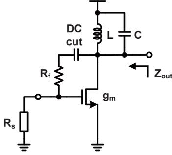
Fig. 2. A resistive feedback amplifier with parallel resonator.
