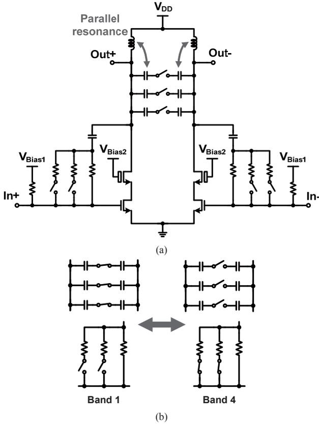
Fig. 3. (a) Schematic of the tunable power amplifier. (b) State of the switches.
