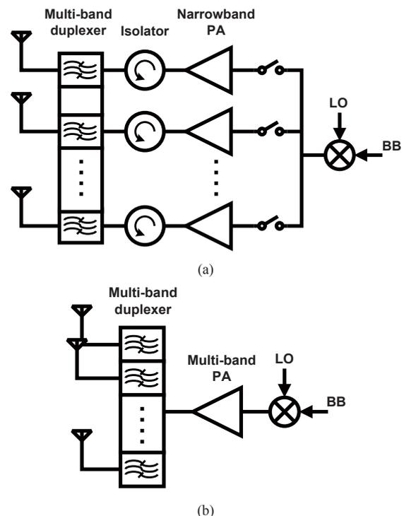
Fig. 1. (a) A conventional multi-band transmitter. (b) The proposed multi-band transmitter.
