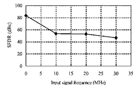
Fig. 1: SFDR versus input signal frequency,  $f_{\text{samp}} = 100$  MHz (taken from [2]).
