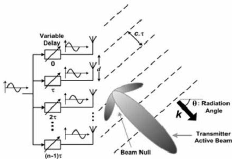
Fig. 1.  $n$ -element phased-array transmitter.
