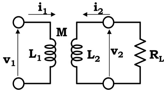
$$P_L = k^2 \frac{L_1}{L_2} I_1^2 R_L \quad k = \frac{M}{\sqrt{L_1 L_2}} \propto \frac{1}{d^3}$$
