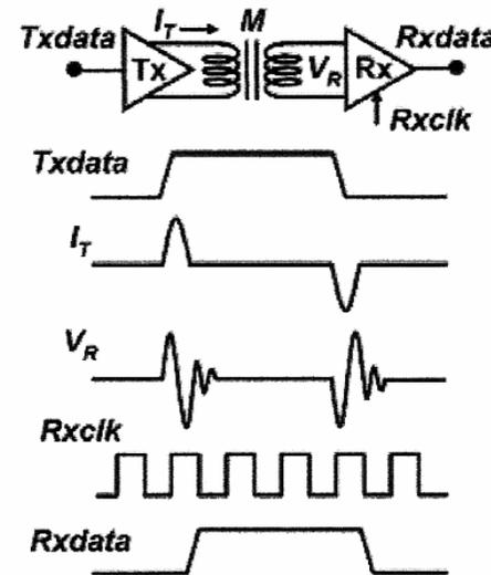
1.2Gb/s/ch, 45mW, 300μm-distance
