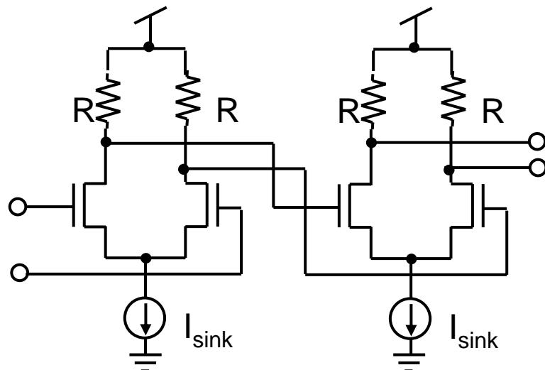
$$GBW = \frac{\mu V_{eff}}{2\pi L^2 \left( \frac{2}{3} + \frac{C_j}{k} \right)}$$
