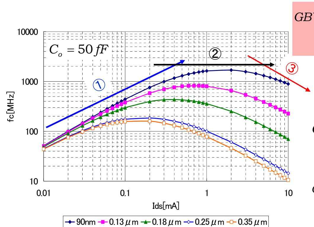
$$GBW_{close} = \frac{g_m}{2\pi C_o} \left( \frac{1}{2 + \frac{C_{pi}}{C_o}} \right) \left( \frac{1}{1 + \frac{C_{po}}{C_o}} \right) + \left( 1 + \frac{C_{pi}}{C_o} \right)$$
