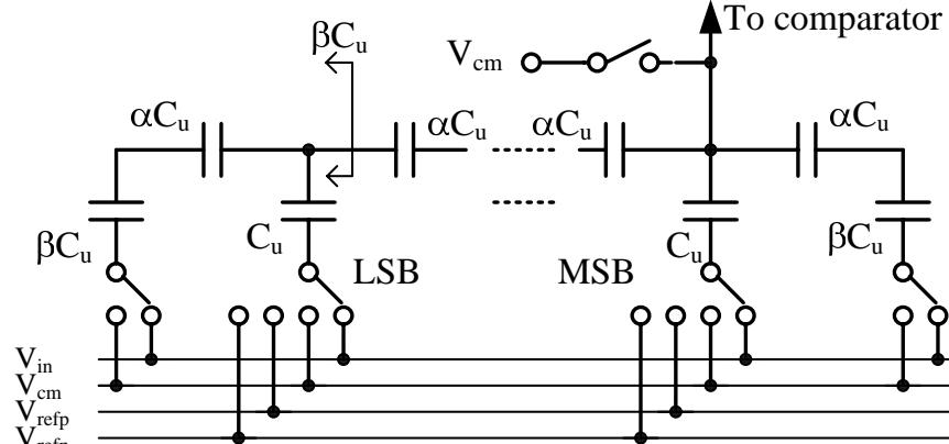
6bit 600MHz 5.3mW ADC has been realized with 0.13um CMOS
