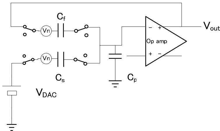
$$G(dB) > 6N + 10 \text{ for 1.5b pipeline ADC}$$
