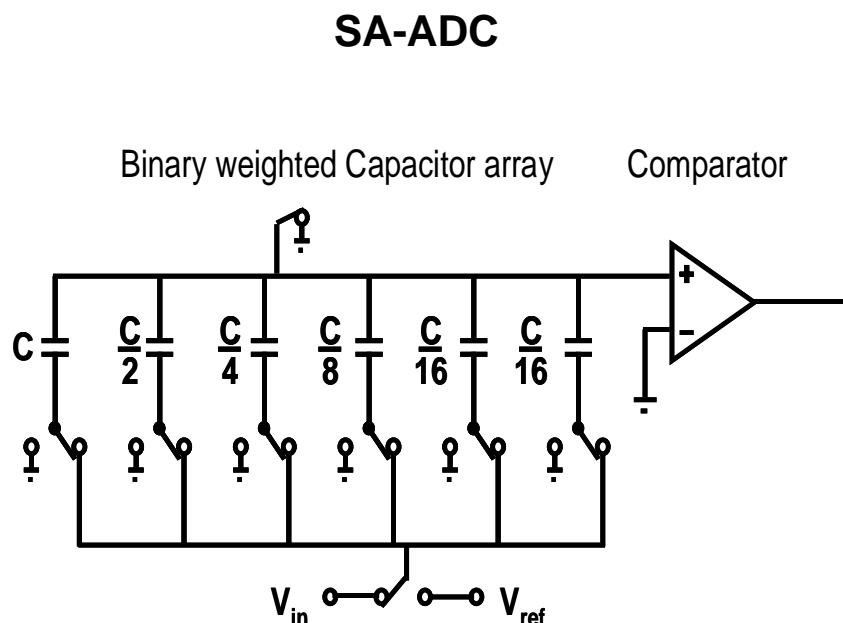
Eight interleaved SA-ADCs with 90nm CMOS attain 600MHz operation.
