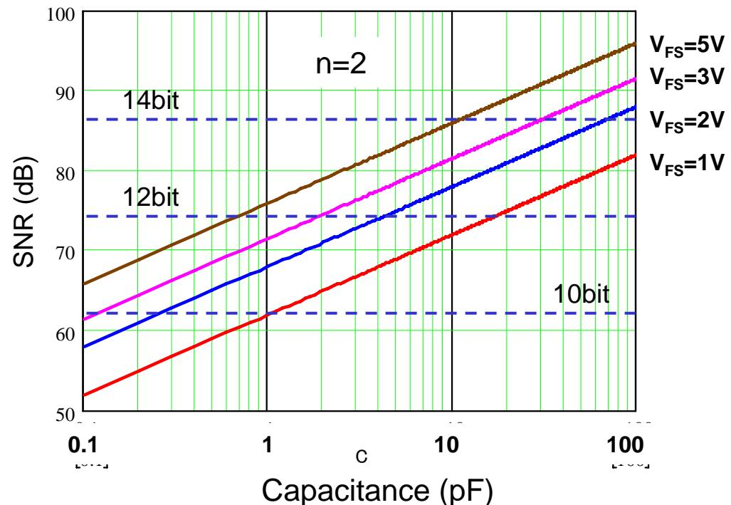
$$\langle v_n^2 \rangle = 4kTR \int \frac{1}{1 + (\omega CR)^2} \frac{d\omega}{2\pi} = \frac{kT}{C}$$
