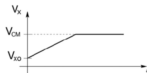
$V_x$  is reaching the virtual ground voltage with constant rate
