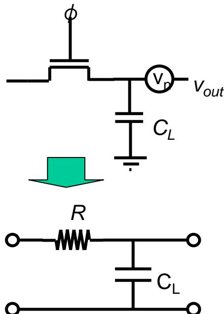
$$\langle v_n^2 \rangle = \frac{nkT}{C} \quad n: \text{configuration coefficient}$$
