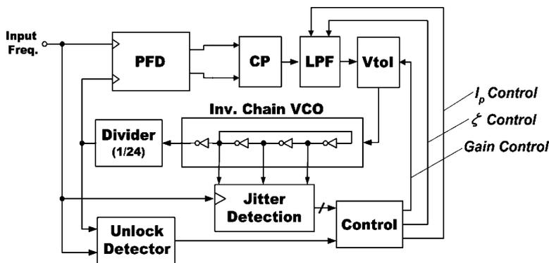
Fig. 2. Block diagram of the PLL with BG calibration.
