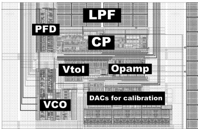
Fig. 14. Layout pattern of the PLL.
