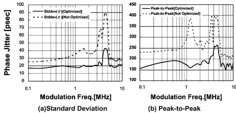
Fig. 16. Jitter performance against the frequency of 10% supply voltage modulation.
