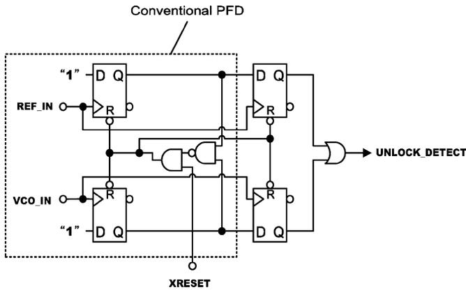
Fig. 9. Schematic of the unlock detector.
