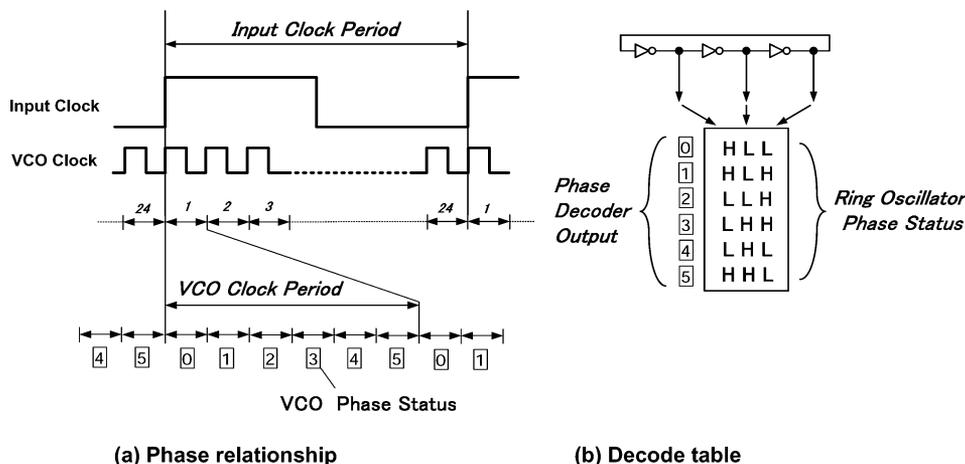
Fig. 3. Concept of jitter detection.
