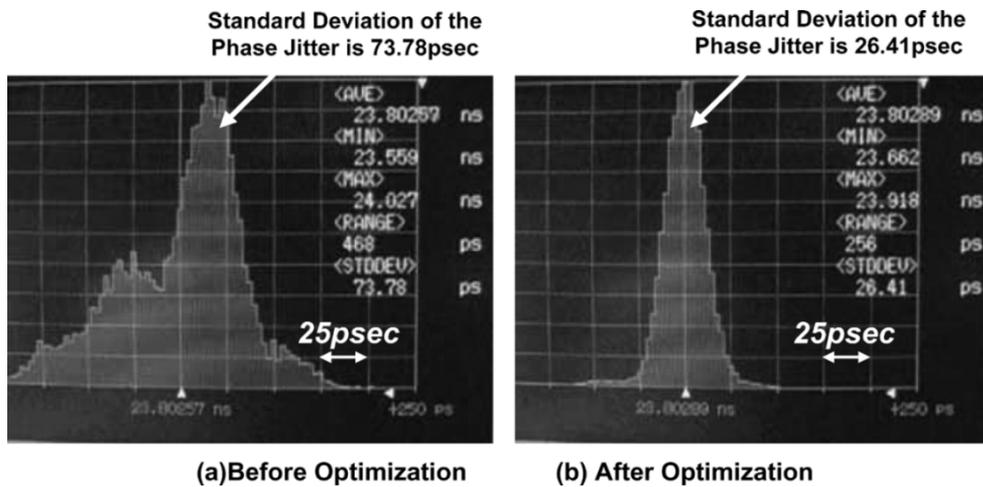
Fig. 17. Comparison of the output jitter spectrum of the TIA (voltage supply noise frequency = 4 MHz).
