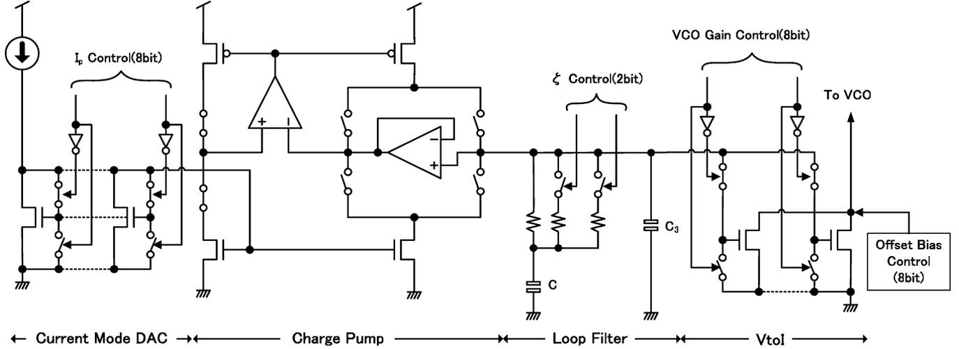
Fig. 6. Schematic of the control for the PLL parameter.
