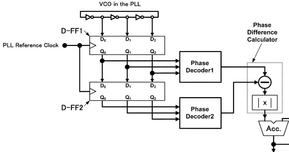
Fig. 4. Block diagram of the jitter detector.
