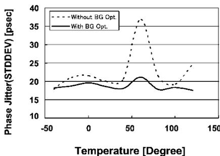
Fig. 20. Comparison of the phase jitter performance against the temperature variation.
