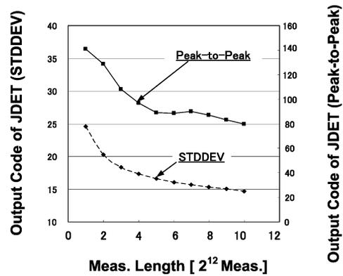
Fig. 15. Statistic values of the jitter detector against the measurement length.
