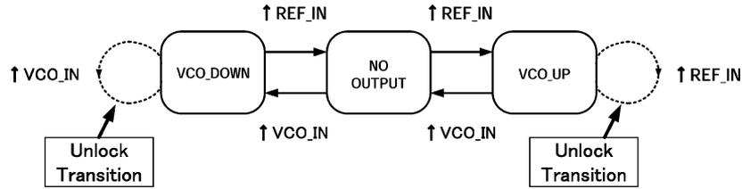
Fig. 8. State-machine diagram of the phase frequency detector.
