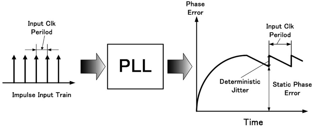
Fig. 7. Mechanism for the generation of the deterministic jitter.
