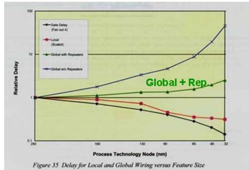
Figure 35 Delay for Local and Global Wiring versus Feature Size
